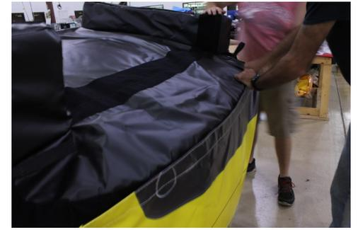
When the cover is secured over the tire blocks, pull the bottom cover over the foam and secure the Velcro of the top cover to the Velcro on the bottom cover. Pull the bottom tight and secure the covers all the way along the seam (above).
