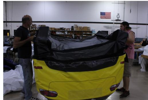
When the cover is secured over the target, flip it over and begin putting the bottom half of the cover on the foam tire blocks.
