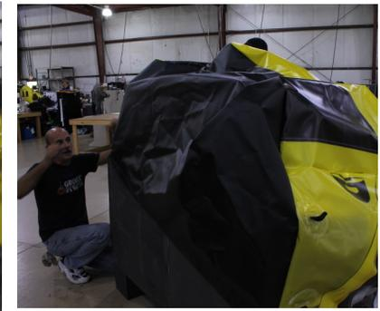
Go to the opposite side of the target and line up the seam of the cover with the edges of the foam target. Slowly pull one side (left or right) down first, and then go to the opposite side and pull the cover down. Try to keep the progression of the cover the same on both sides.
